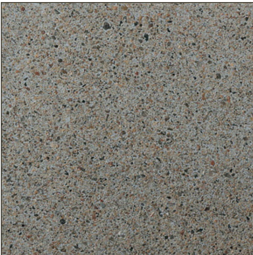
Acid Washed Concrete
